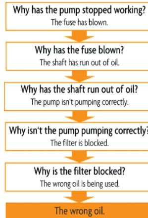
imperative: in this case, the cause of the oil pump malfunction is the use of the wrong oil. This has blocked the filter, preventing the pump from pumping correctly and starving the shaft of oil, which has then overheated and caused the fuse to blow. Identifying the root cause of a chain of faults and addressing it (in this case, by administering the correct oil) means that symptoms are unlikely to recur.
